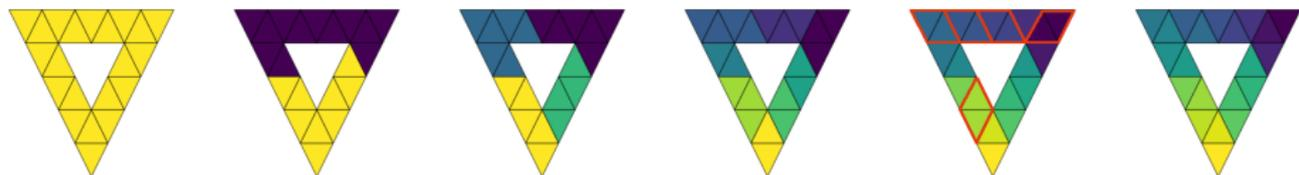
A synthetic simplicial complex with  $k = 2$ . Successively bipartitioning the subcomplexes induced by prior partitions leads to finer, nicely localized domains, illustrated by piecewise-constant functions on the triangles. Proceeding left-to-right, each complex has been bipartitioned to one finer level.
